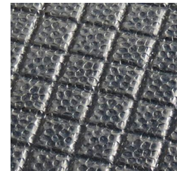
rhombic profile with top coat
